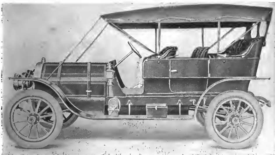
MODEL 75, GEARLESS, HAS SIX-CYLINDER, FOUR-CYCLE MOTOR.
